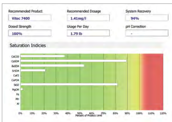
FIGURE 1. Scaling model, 94% recovery with Vitec 7400 at TDS = 2,700 mg/L.
